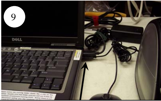
9 Plug Dymo cable into Right side of PC.
