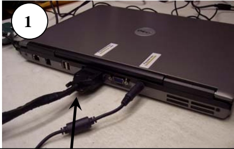
Connect the autorefractor serial cable.
