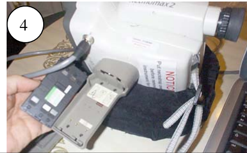
Align battery with 3 button side down
