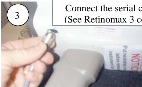
Align black mark on case to black mark inside connector.
